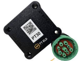
**Step 3:** Connect the ELD plug to the diagnostic part of the vehicle. Unscrew the lock surface until it locks. Make sure the ELD is connected
